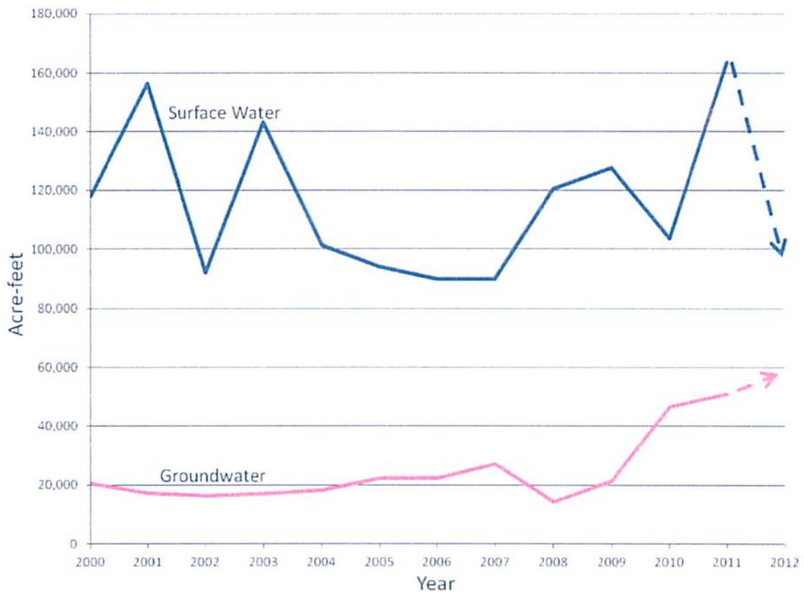
Figure 5. Usage of surface water (top line) and groundwater (bottom line) for irrigation in Colorado County from year 2000 through 2011. Dashed lines indicate projected trends beyond 2011. Modified from data provided in Appendix C1 (Allen, 2014; TWDB 2014).
