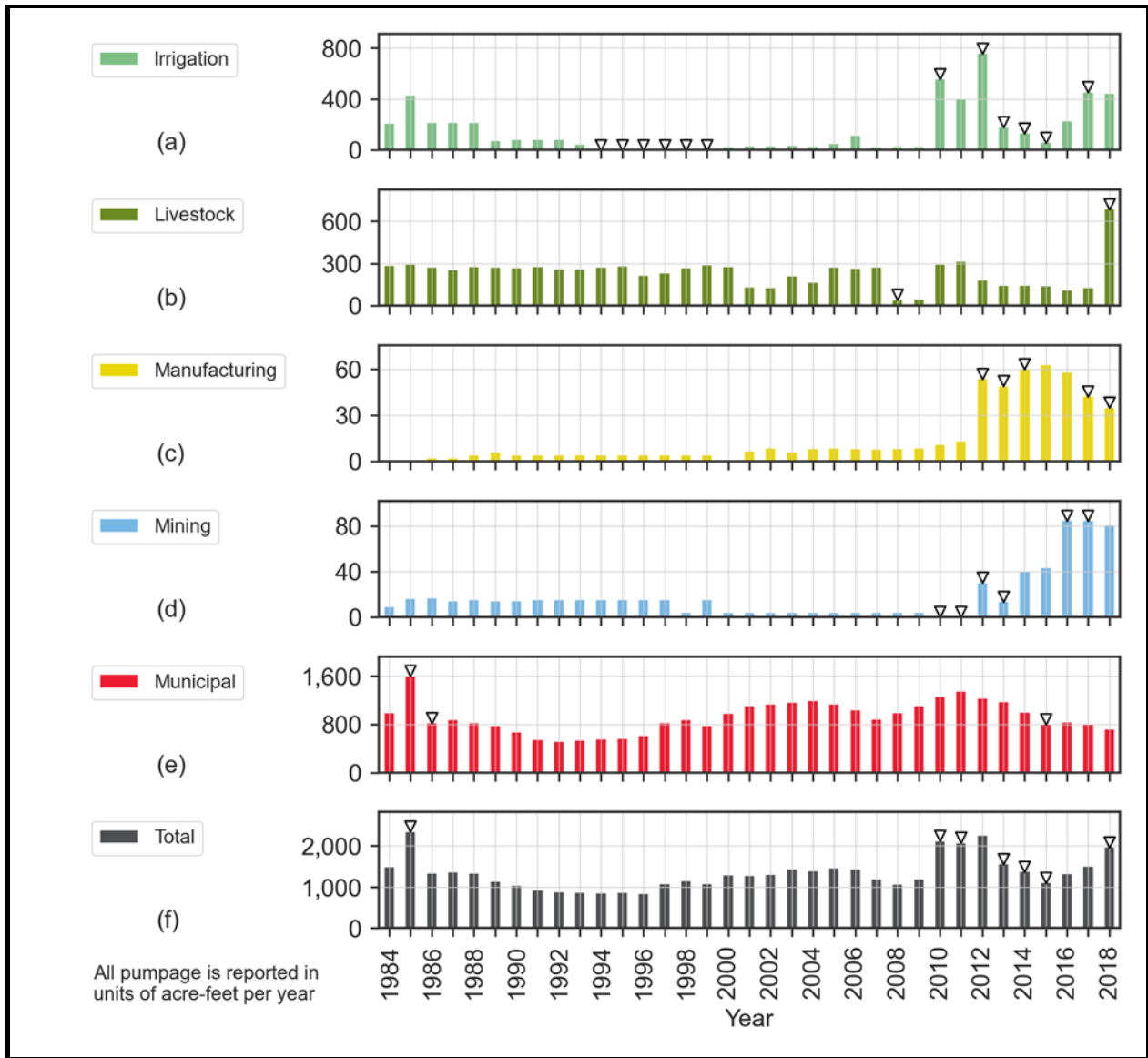
Figure 60. Burnet County Trinity (Hill Country) Aquifer apparent anomalies based on the criterion of 1.5 standard deviations from the 3-year average of groundwater pumping in acre-feet per year as reported in the TWDB Water Use Survey data. Triangles mark years where the data appears anomalous.
