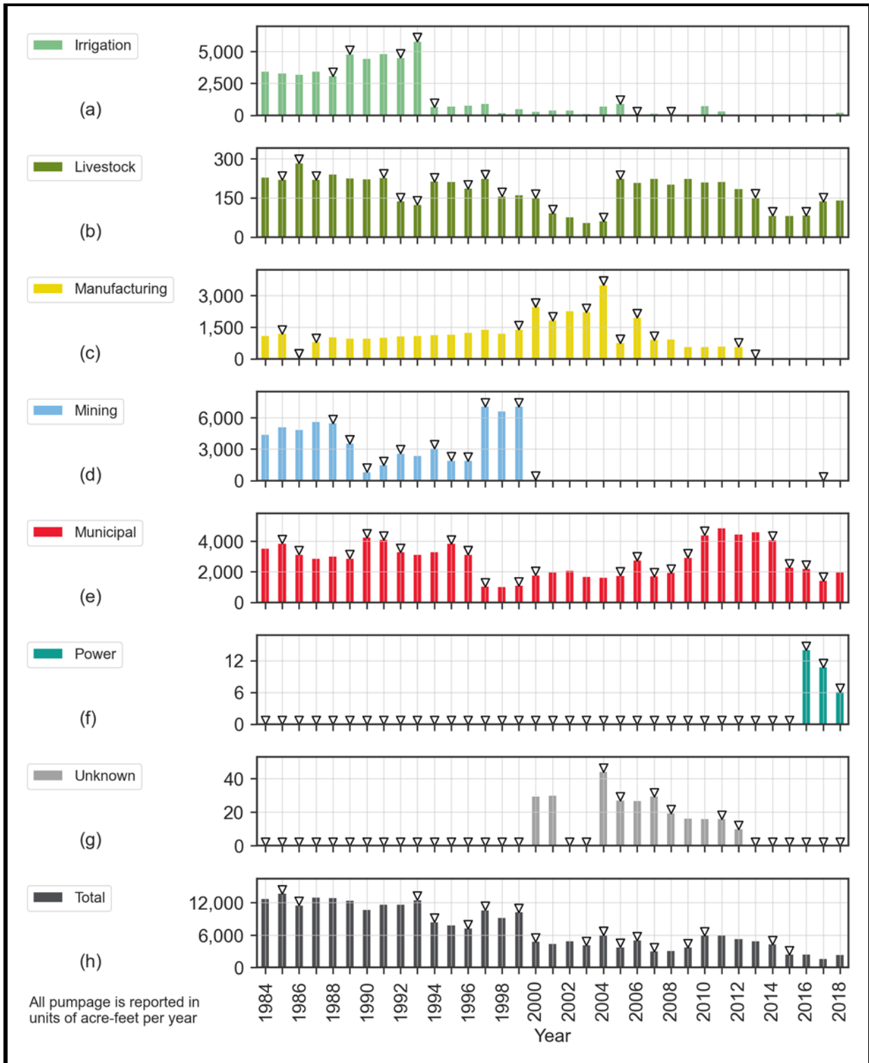
Figure 113. Ector County Edwards-Trinity (Plateau) Aquifer apparent anomalies based on the year-to-year change in groundwater pumping in acre-feet per year as reported in the TWDB Water Use Survey data. Triangles mark years where the data appears anomalous.
