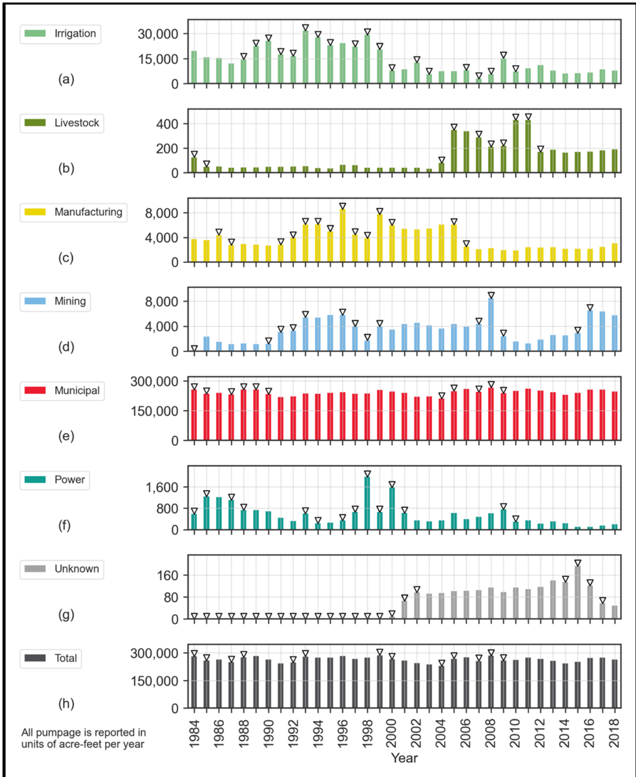
Figure 39. Bexar County Edwards (Balcones Fault Zone) Aquifer apparent anomalies based on the year-to-year change in groundwater pumping in acre-feet per year as reported in the TWDB Water Use Survey data. Triangles mark years where the data appears anomalous.
