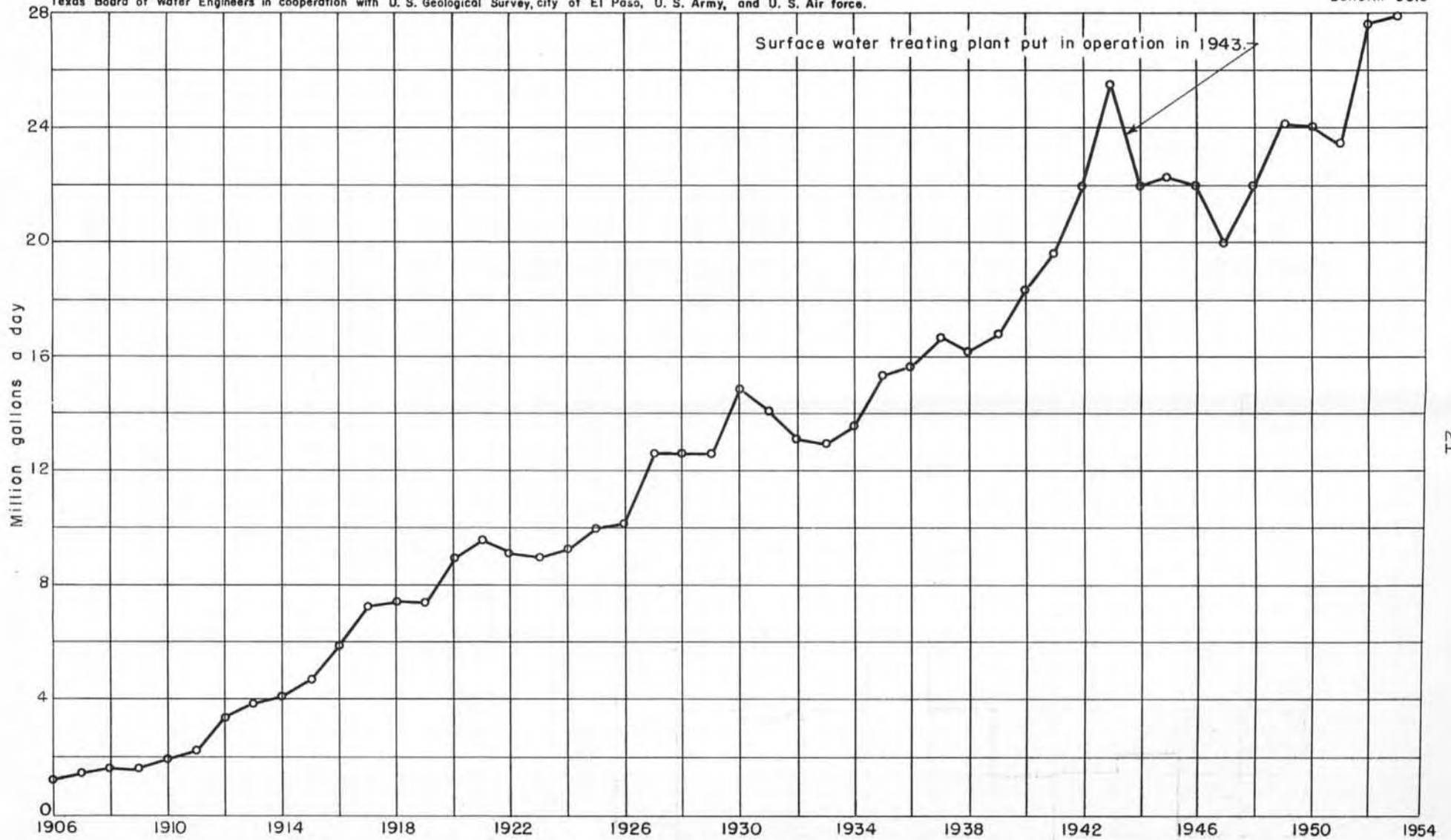
FIGURE 7. - Estimated average daily pumpage from all deep wells (except irrigation wells) in the El Paso area, Tex., 1906-53, inclusive
