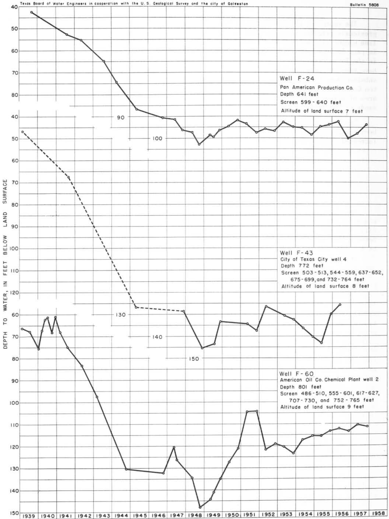
FIGURE 9. - Changes in water level in wells in the sands of the upper part of the Beaumont clay, Texas City area, Galveston County, Tex.
