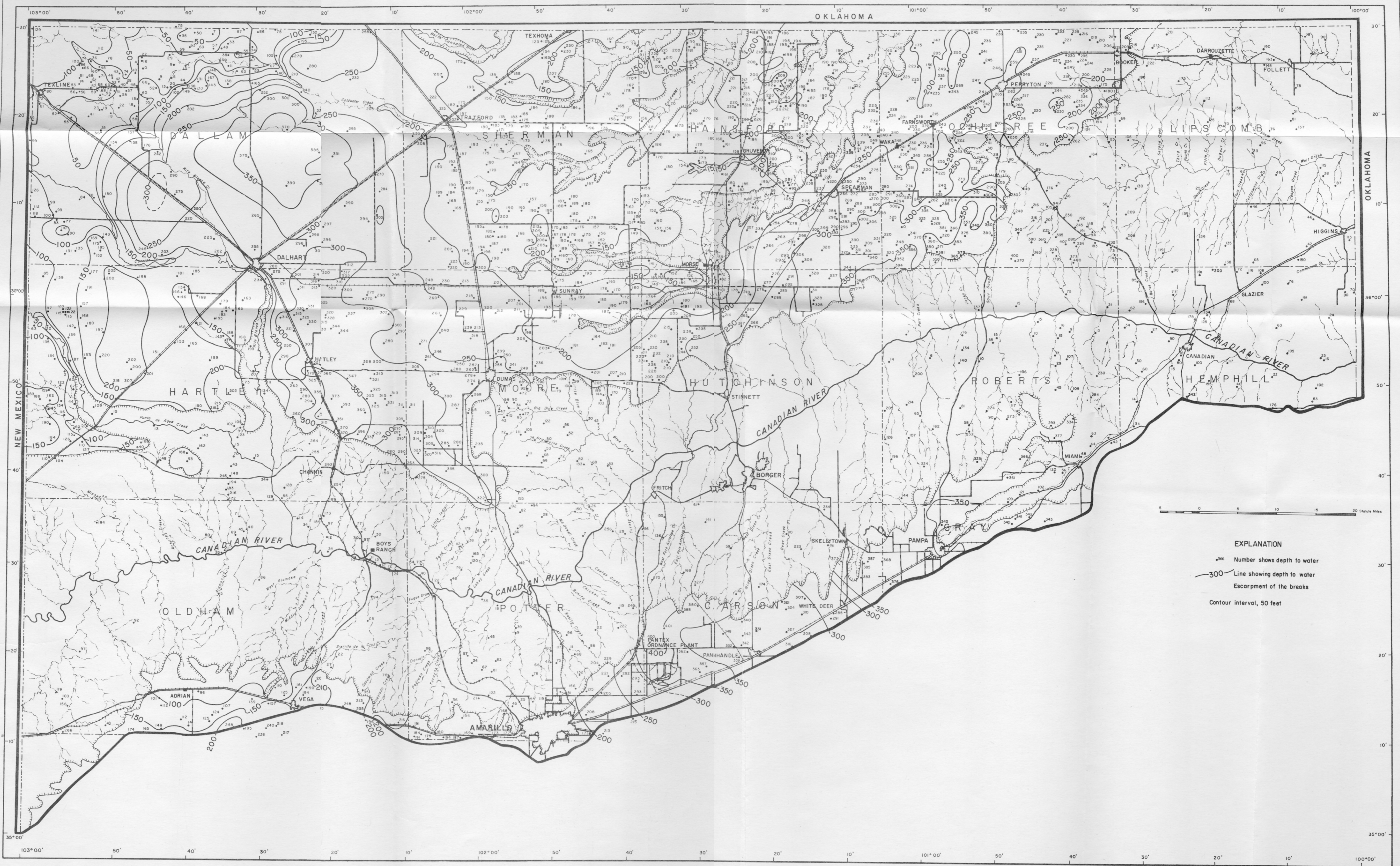
MAP SHOWING DEPTH TO WATER BELOW LAND SURFACE, CANADIAN RIVER BASIN, TEXAS 1959
