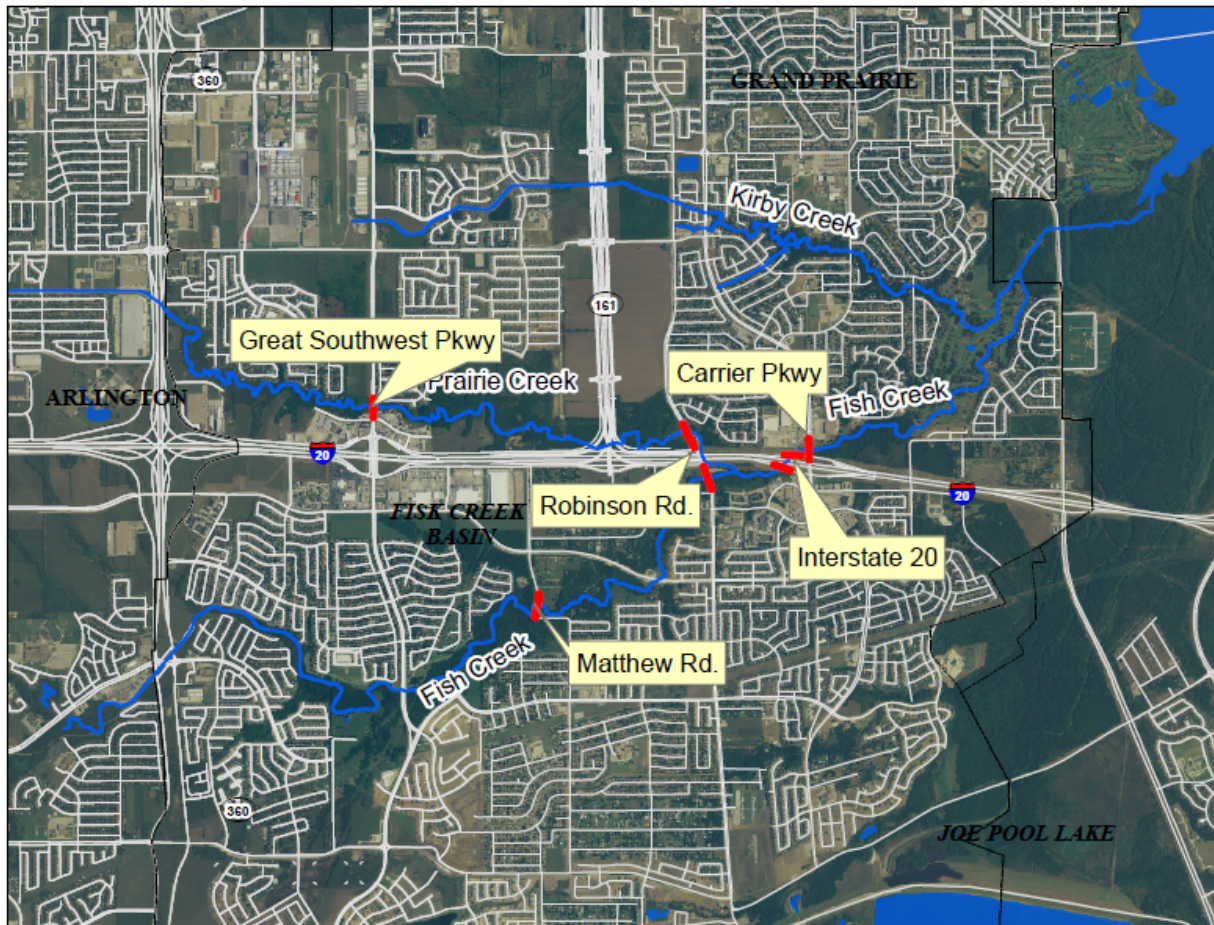
Figure 10: Fish Creek Basin Bridges Overtopped by a 100-YR Storm
