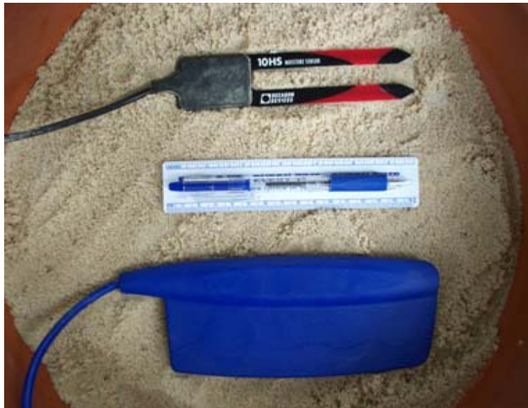
Soil Moisture Sensors – Echo (upper device) and Aquaspy (lower device)
