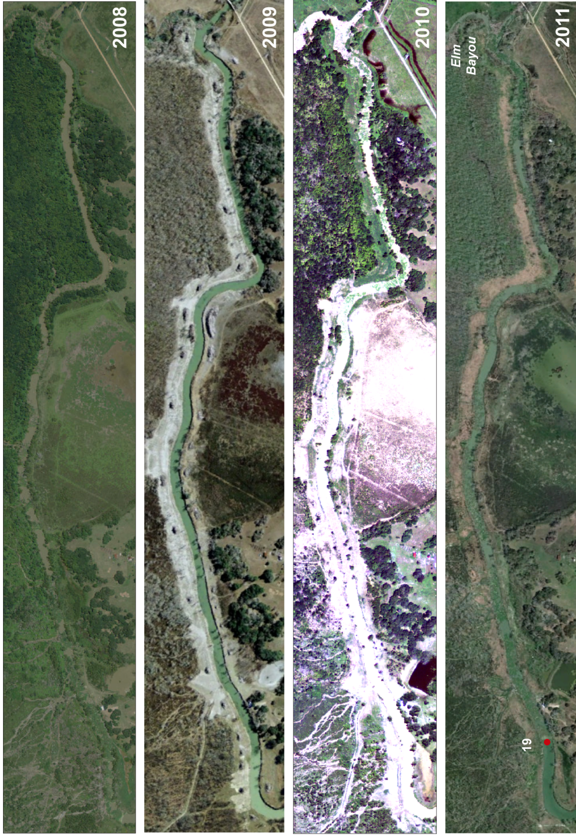
Figure 6. Accumulation of large woody debris in subreach 19. Flow direction is from left to right. The upstream limit of the subreach is indicated by numbered circle on the 2011 image.
