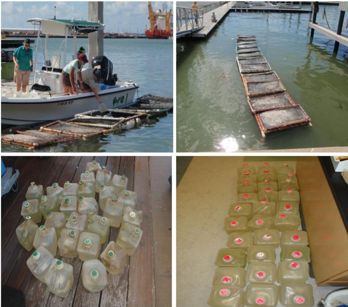
Fig. 3 Experimental set up - each sample was incubated at ambient water temperatures, turbulence and under 50% ambient sunlight in an outdoor facility at TAMUG. At the end of the experiment the 180 cubitainers are retrieved and processed in the laboratory.
