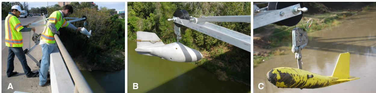
Figure 3.1: Primary sampling equipment. (A) US DH-2TM bag-type sampler suspended from the sampling crane; (B) US BMH-60 bed material sampler; and (C) sounding weight.
