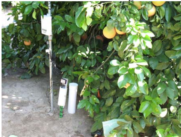
Below: WatchDog data logger and WaterMark soil moisture sensor installation next to Decagon ECH 2 O soil water monitoring equipment on Collaborator #01's farm to help facilitate soil moisture readings for farmer.
