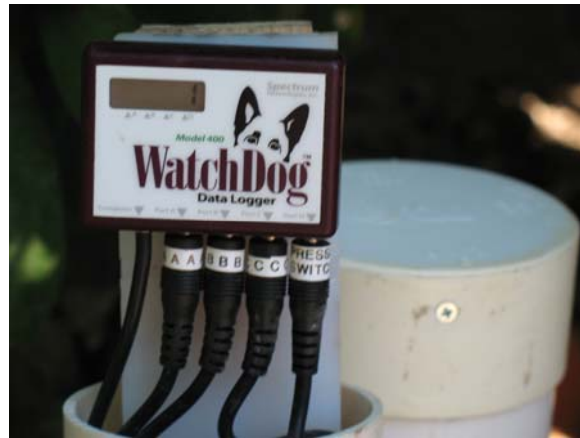
Below: WatchDog data logger and WaterMark soil moisture sensor installation next to Decagon ECH 2 O soil water monitoring equipment on Collaborator #01's farm to help facilitate soil moisture readings for farmer.
