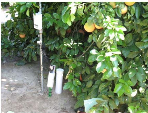
Above: ADI collaborator #01 has mature Rio Red grapefruit and Valencia oranges on this plot. WatchDog data logger was installed to help facilitate soil moisture readings for farmer.
