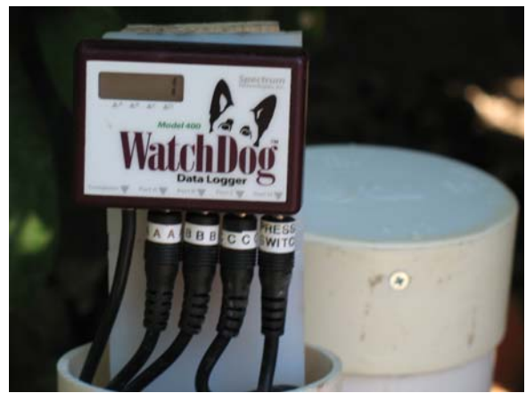
Above: ADI collaborator #01 has mature Rio Red grapefruit and Valencia oranges on this plot. WatchDog data logger was installed to help facilitate soil moisture readings for farmer.
