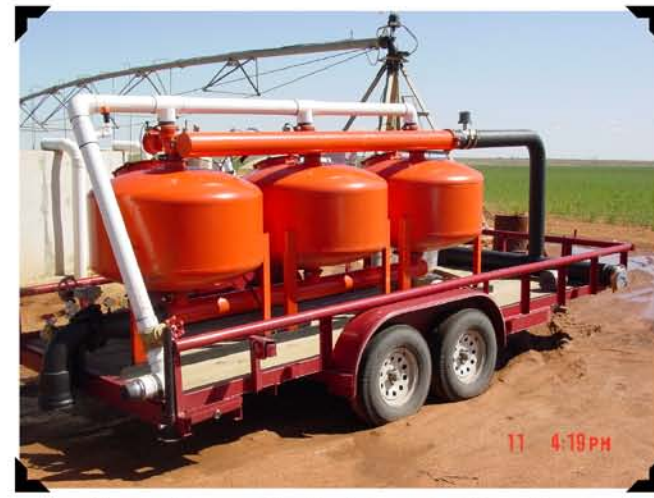
Filter system used in the drip project for cotton.
