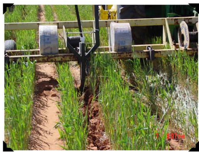
Closeup of tape as it is plowed into the field.
