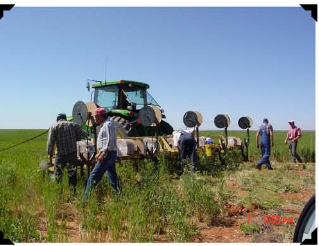
Tractor with 5 reels attached to a toolbar
