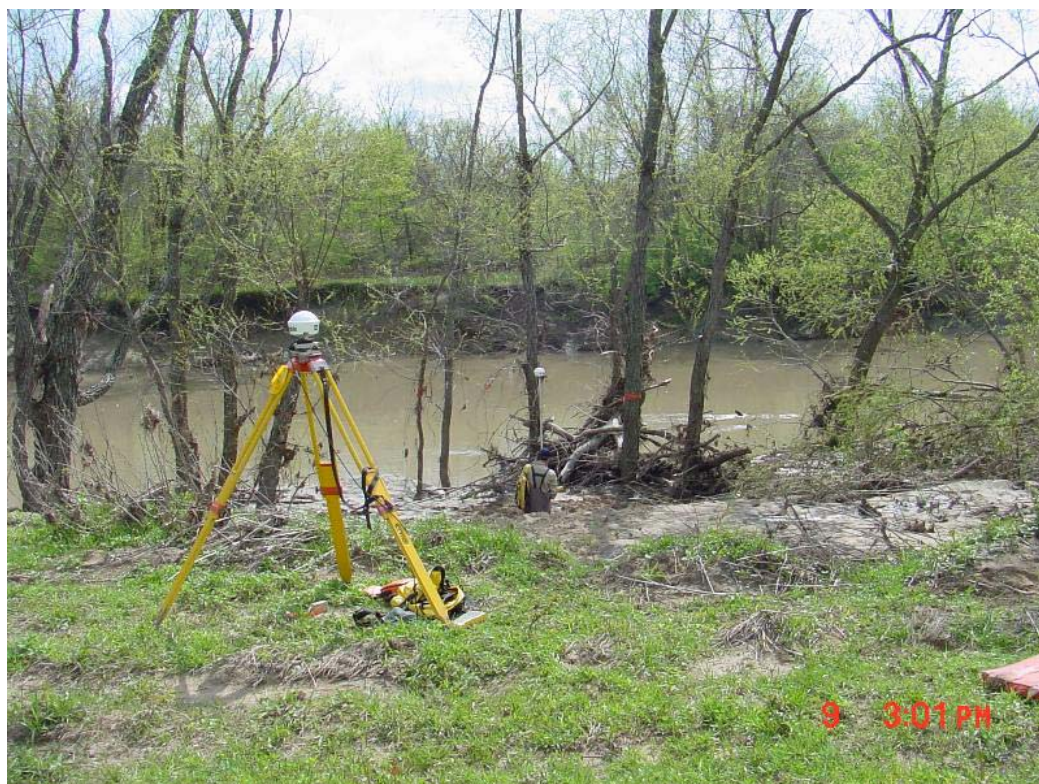
Figure 6.7– Photo of inundation in channelized section at high flow at upstream boundary of Site 1, downstream of the confluence, April 9, 2002 (342.6 cms, 12,100 cfs at Talco).
